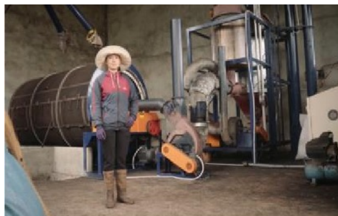
Pyrolysis system with drum dryer (left) manufactured by Viet Hien Co. and implemented at Binh Minh Cooperative
